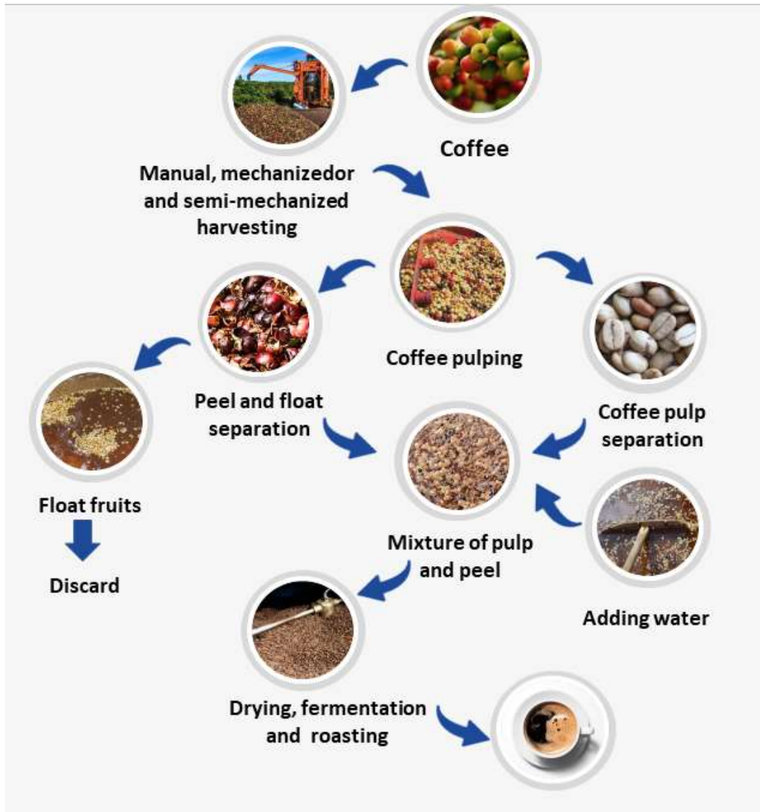
Figure 5. Schematic representation of coffee processing by the wet method.
