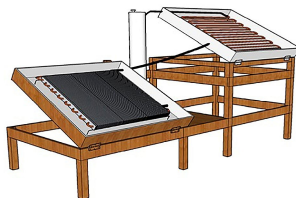
Figure 1: Schematic representation of the Sandwich Solarizer (STS) model. Source: José Roberto Vieira Junior – Embrapa Rondônia.
