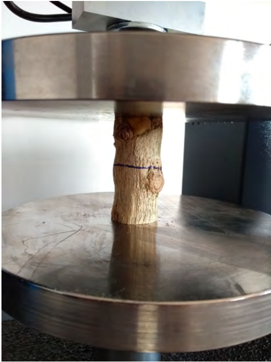
Figure 5: Specimen produced from the trunk of a coffee plant sample being subjected to compression testing, in a universal testing machine, in the direction parallel to the fibers.
