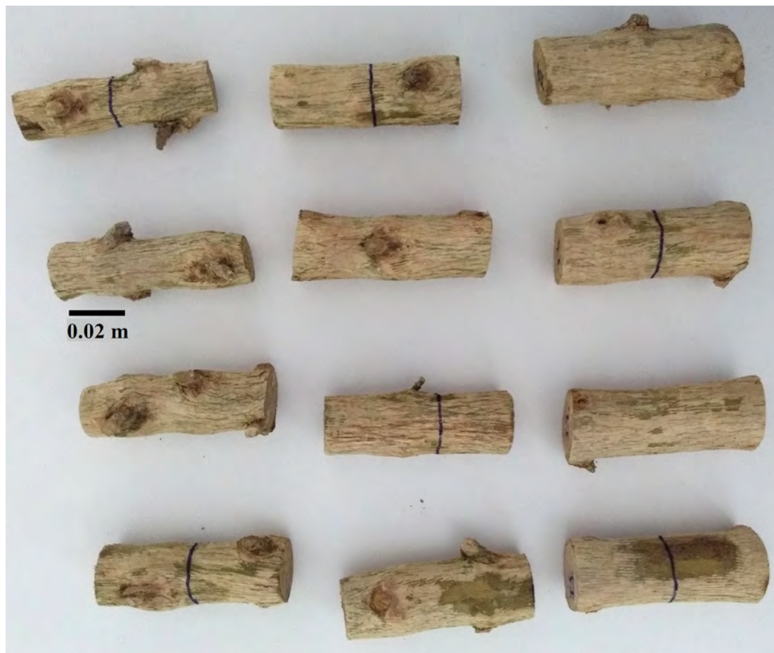
Figure 1: Specimens produced from the trunks of a coffee plant sample and which were subjected to compression tests in the universal testing machine, in parallel and perpendicular to the fibers.
