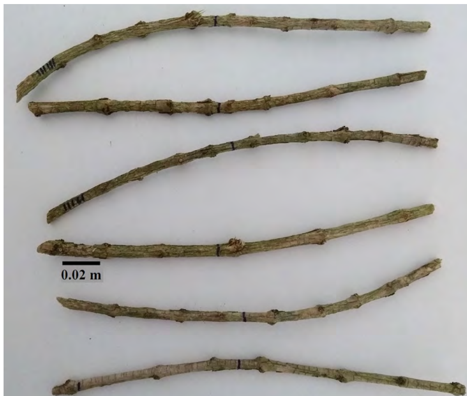
Figure 3: Specimens produced from the branches of a coffee plant sample and subjected to tensile tests, in a universal testing machine, in the direction parallel to the fibers.
