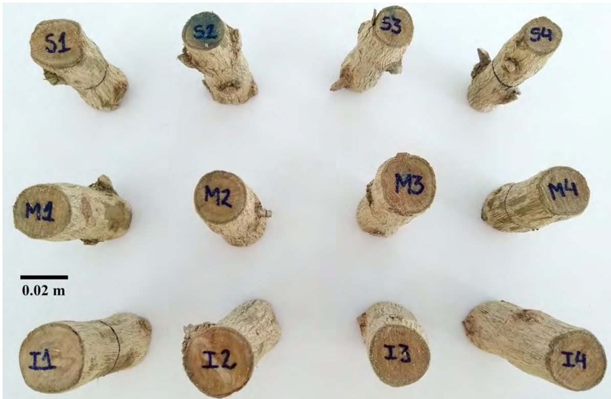
Figure 2: Identification in each specimen produced from the trunks of the coffee plants, which were subjected to compression tests in a universal testing machine, where S refers to the upper third, M to the middle third and I to the lower third.
