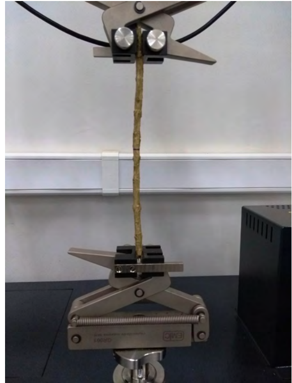
Figure 7: Specimen produced from the branch of a coffee plant sample being subjected to tensile testing, in a universal testing machine, in parallel direction to the fibers.
